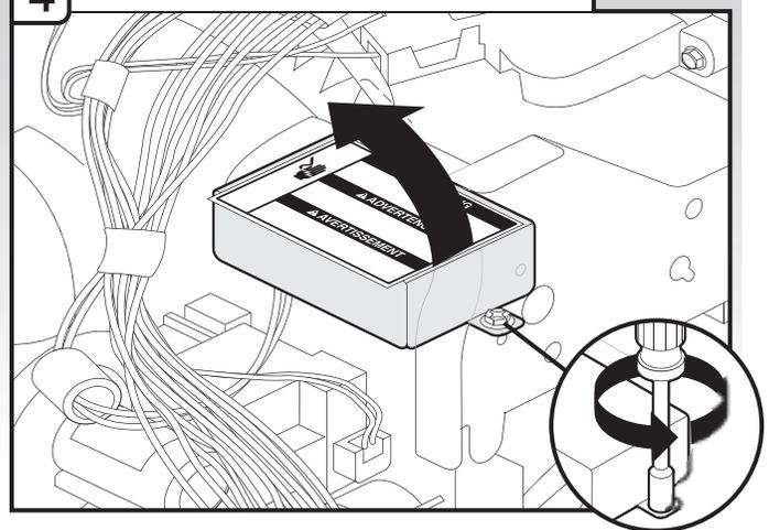
Using a 1/4" hex head socket, nut driver or Phillips screwdriver, remove terminal box cover. Retain for later use.
